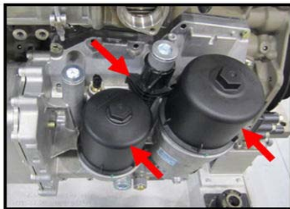
New lock: STD1534PE no repair necessary
