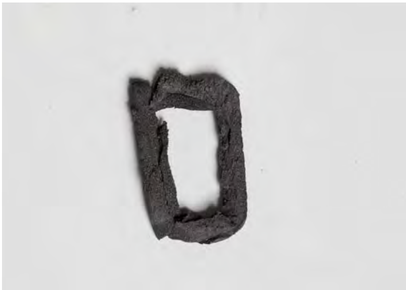
Figure 27 Typical Condition of the Foam Seal after Removal
