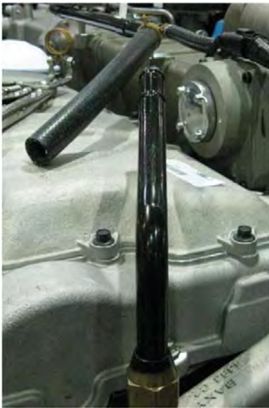
Figure 21 Aligning Heater Supply Tube
