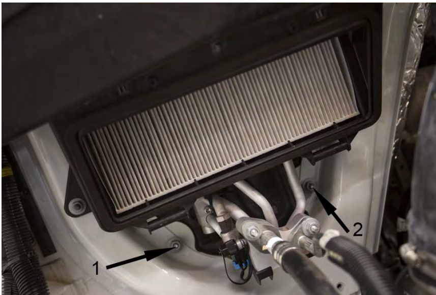
Figure 25 Loosening Mounting Nuts
