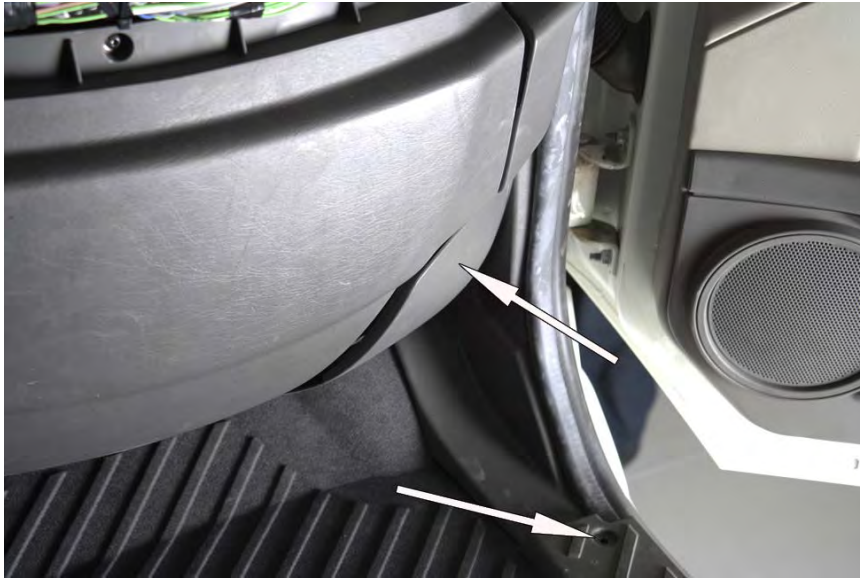
Figure 22 Removing Kick and Scuff Panels
