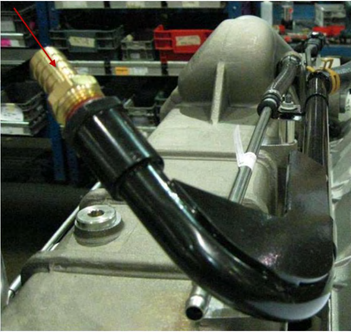
Figure 19 Adding Nipple to Assembly Heater Front Supply Pipe
