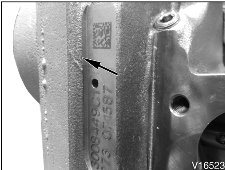
Figure 10 EGR Housing Surface Height Difference
