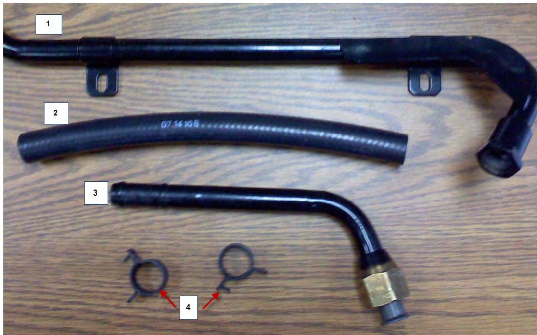
Figure 18 Three-Piece Heater Supply Hose
