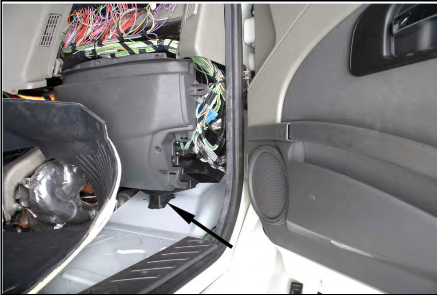
Figure 24 Pulling Floor Mat away from Drain Area
