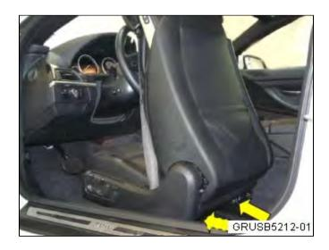
1. Move the front seat fully forward to expose both rear nuts securing the seat mechanism to the seat rail.
