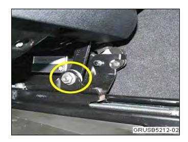
height setting and the most forward backrest setting to reveal the securing nuts. Shown is the driver's side nut on the tunnel side.
