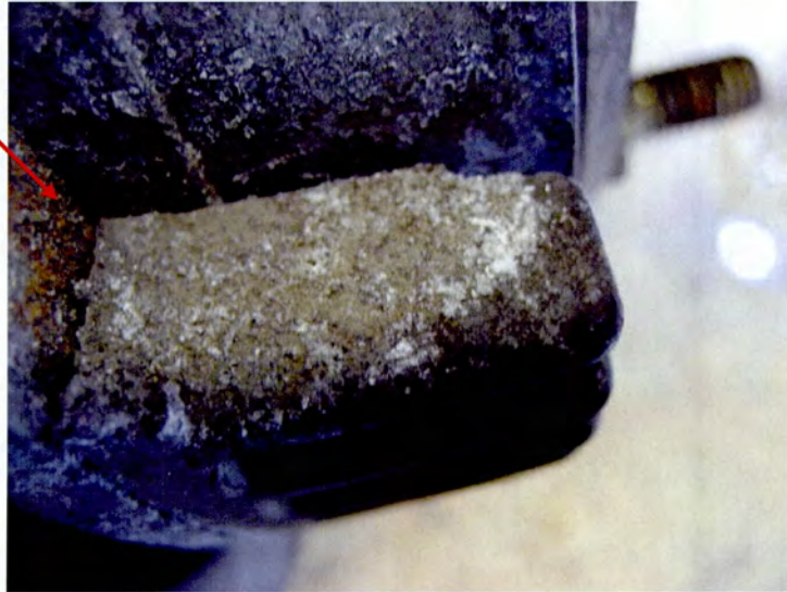
Figure 3: Exhibits missing portion of the cooling ring
