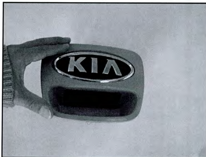
A sample of "manual release type" outer handle
