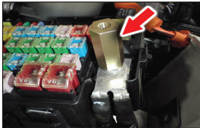
FST9001 - Battery Charging Terminal Adaptor (red arrow) installed on the B+ post in the PDC.
