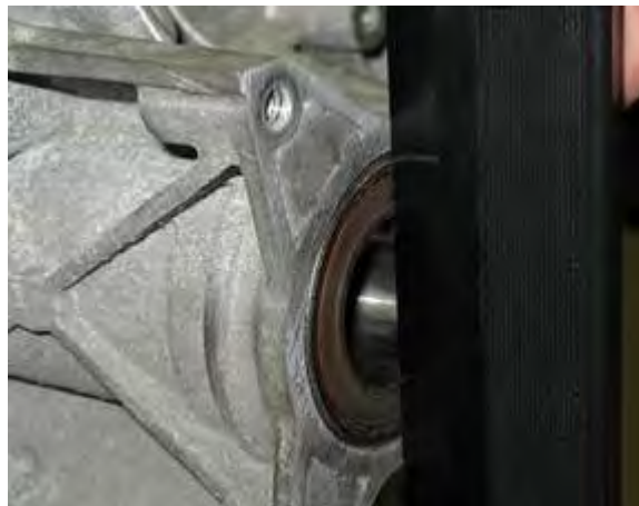
Figure 5. Apply straightedge on gearbox housing/bearing.
