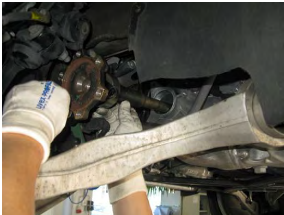
Figure 3. Pulling out the flange shaft.
