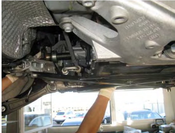
Figure 2. Supporting the flange shaft.
