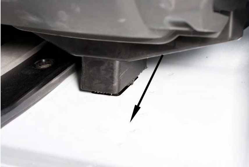
Figure 21 Pulling the HVAC Unit Rearward
