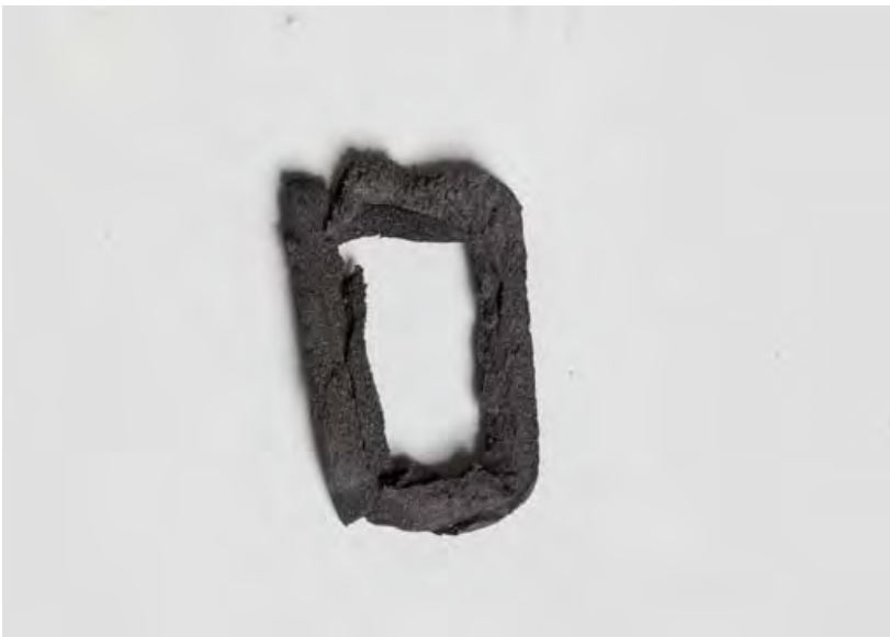
Figure 22 Typical Condition of the Foam Seal after Removal
