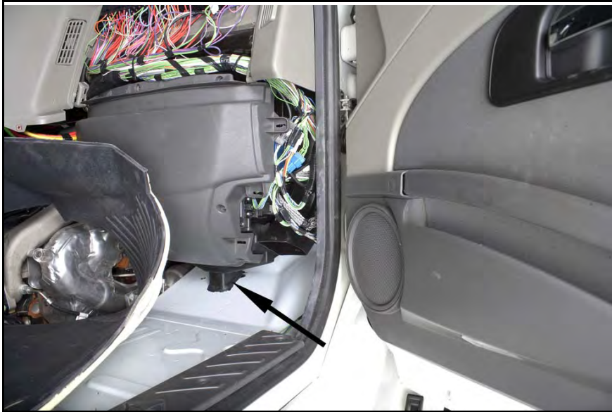
Figure 19 Pulling Floor Mat Away from Drain Area
