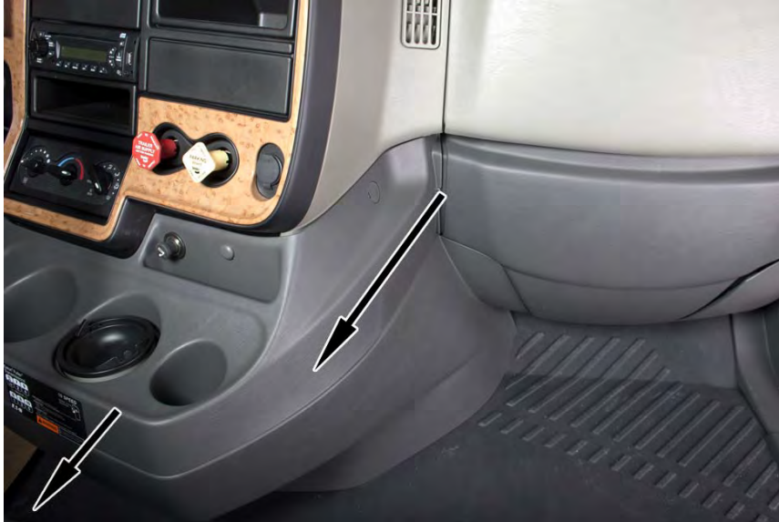
Figure 2 Detaching Center Console
