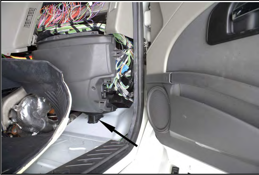
Figure 3 Pulling Floor Mat away from Drain Area
