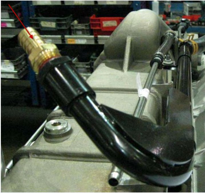
Figure 3 Adding Nipple to Assembly Heater Front Supply Pipe
