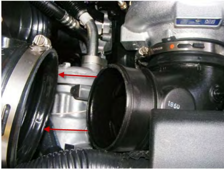
Figure 1 Removing tube from inlet boot
