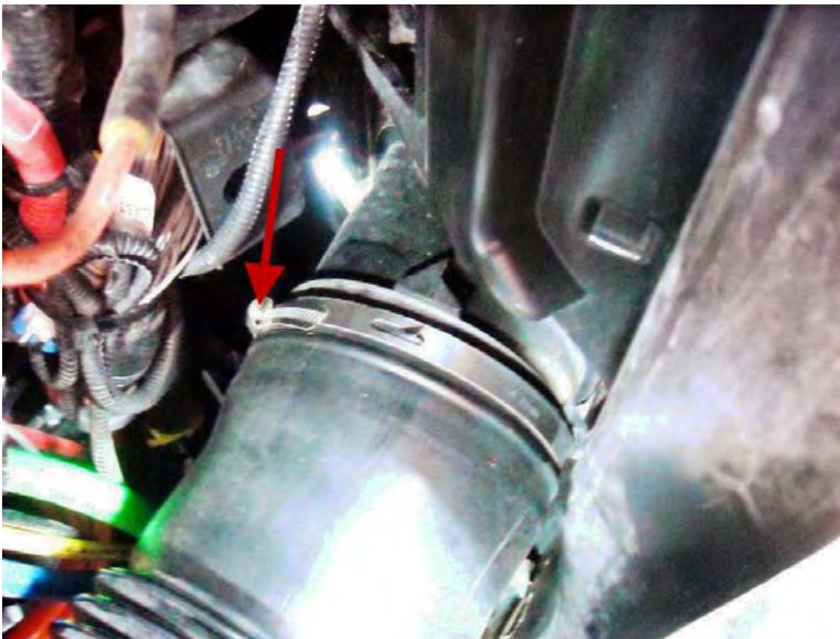
Figure 2 Air intake pipe clamp location
