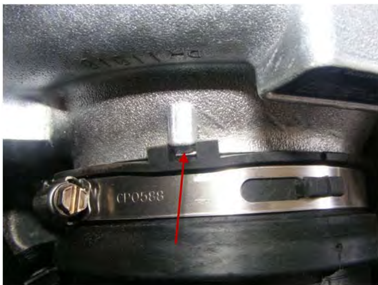
Figure 3 Turbocharger alignment notch
