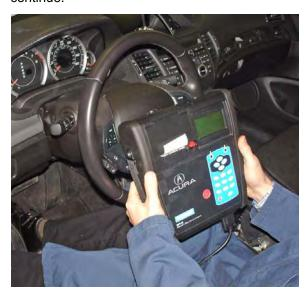
17 When prompted, turn the ignition switch to ON (I). Make sure all electrical loads are off at this time.
