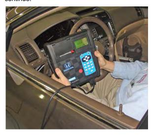
17 When prompted, turn the ignition switch to ON (I). Make sure all electrical loads are off at this time.
