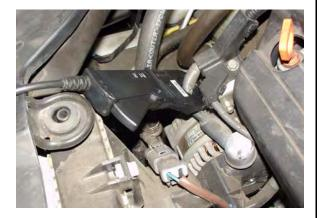
16 Remove the control module from the top of the GR8, and take it into the vehicle. Press NEXT to continue.
