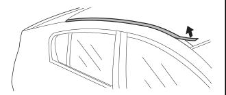
5. At the rear of the molding, pull up and release the rear bracket from the pin.
