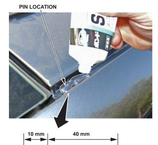
9. Reinstall the roof molding immediately after applying the Konishi Bond.
