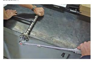
22. Before installing the new VTC actuator, make sure it is in the unlocked position.
