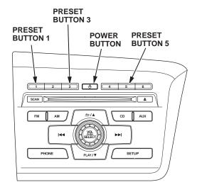
After about 5 seconds, the audio unit software version screen appears. Release the buttons. The version should be SYS1100.
