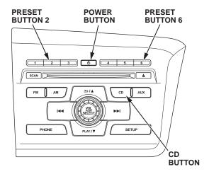
After about 5 seconds, the A-DIAG DOWNLOAD screen appears. Release the buttons.
