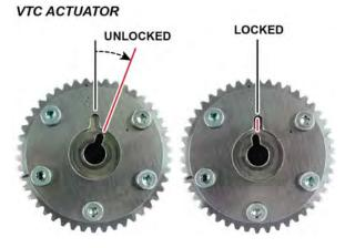
23. Install the new, unlocked VTC actuator onto the camshaft; do not force it on.
