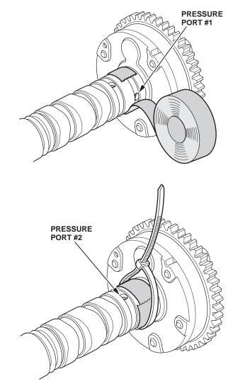
27. Apply compressed air to pressure port #2. While air pressure is applied.to pressure port #2, rotate the VTC Actuator by hand in the direction shown (as needed) to unlock the VTC Actuator.
