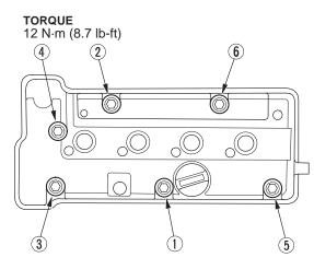
46. Reinstall the EVAP canister purge valve bracket.
