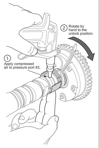
Verify the actuator has moved to the unlock position.
