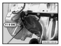
8. Install the locating pin (Special Tool 11 9 590) to lock the position of the engine.
