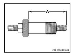
11. Remove the chain tensioner Special Tool 11 9 340 from the engine, with the lock nut still tight. Measure the distance (A), as described in the illustration.
