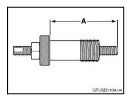
11. New Remove the chain tensioner Special Tool 11 9 340 from the engine, with the lock nut still tight. Measure the distance (A), as described in the illustration.
