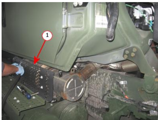
Image 2 - Remove Right top Step Heat Shield - 4 bolts
