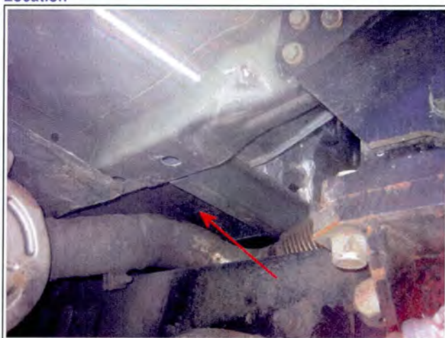
Photo 1 - Cab Floor Insulator Location - Right side
