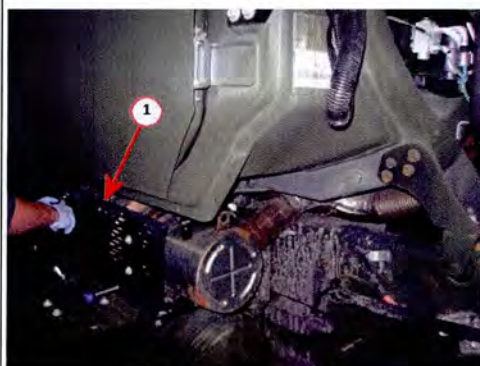
Image 2 - Remove Right top Step Heat Shield - 4 bolts
