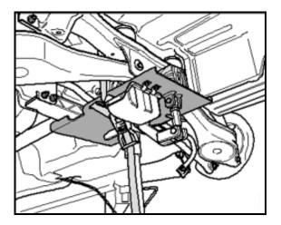
Support rear axle with an engine/transmission jack
