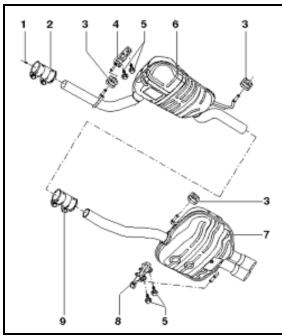
Remove rear exhaust -7- by removing bolts -5- for exhaust hanger -8- and disconnect from retaining loop -3-
