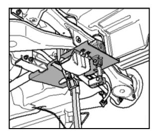
Support rear axle with an engine/transmission jack V.A.G 1383 A with universal support plate V.A.G 1359/2 below subframe and secure with strap
