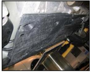
Remove sound dampening trim (pictured) on driver side to expose positive battery cable
