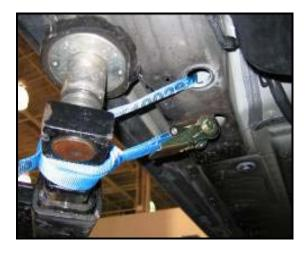
Install special tool T10038 (or equivalent) on driver side rear and passenger side rear to secure vehicle on hoist
