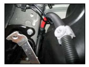
Route cable along brake lines, corrugated harness and fuel tank
