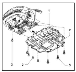
Remove noise insulation cover -1- by removing screws -2- and -3- (if equipped)
