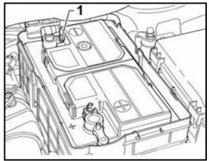
Reconnect battery terminal of ground cable -1- on negative battery terminal and torque to 6 Nm
