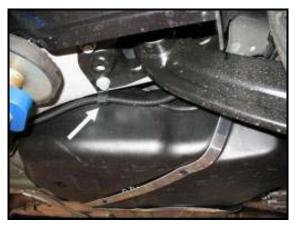
Secure corrugated harness -arrow- (cable for regulator motor of brake caliper housing) back into position
