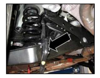
Carefully route the new positive battery cable via the rear axle
