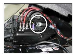
Open cap of the fuse box and remove retaining nut -circle- for the positive battery cable
