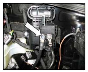
Open cap of jump start junction block and remove retaining nut for the positive cable -arrow-
