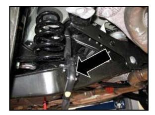
Carefully route new positive battery cable via the rear axle
