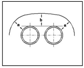
Align rear exhaust system so that distance -a- right and left are equal; then, proceed to Section E
