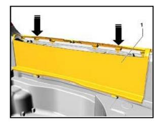
□ Reinstall lock carrier cover -1- downward and onto lock carrier
