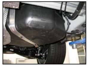
Detach fuel tank securing strap on driver side and loosen strap on passenger side to allow fuel tank to lower slightly
