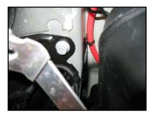
Route cable according to its original routing and clip properly in place
