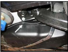
Unclip corrugated harness -arrow- (cable for regulator motor of brake caliper housing)
