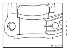
Acceptable camshaft bearing ledge – minor gray wear marks from the rotation of the camshaft are normal. If deep groves are not apparent, the camshaft bearing ledge is acceptable and should not be replaced.
