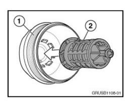
2. New The oil filter cap insert may have been inadvertently removed during the vehicle's last oil service. If this insert is not installed, it will result in non-filtered engine oil being supplied to the engine, thus possibly clogging or damaging the VANOS solenoids.
