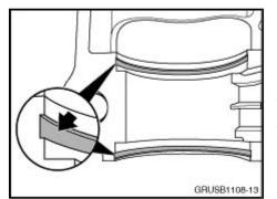
Note the deep grooves worn into the camshaft bearing ledge by the camshaft hook ring seals. The camshaft bearing ledge is worn.
