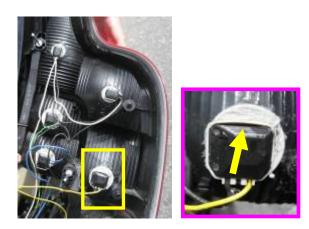
Remove the tail lamp and inspect the bulb holder to ensure the harness alone will repair.
