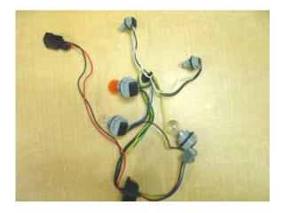
Harness only. Be sure to align the lamps to their correct position. Use the original harness and/or VIDA for reference.
