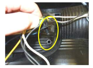
Be sure to reinstall the clip holding the harness to the lamp assembly.
