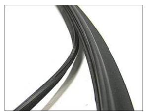
Wiper blade torn or insert separated.
