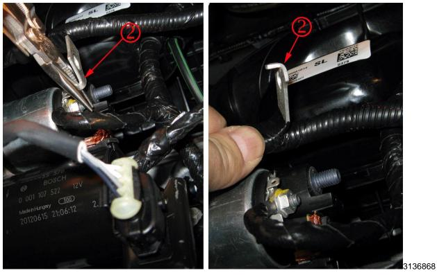
5. Using pliers bend the positive battery cable terminal tab (2) 90 degrees inward as shown in illustration.
