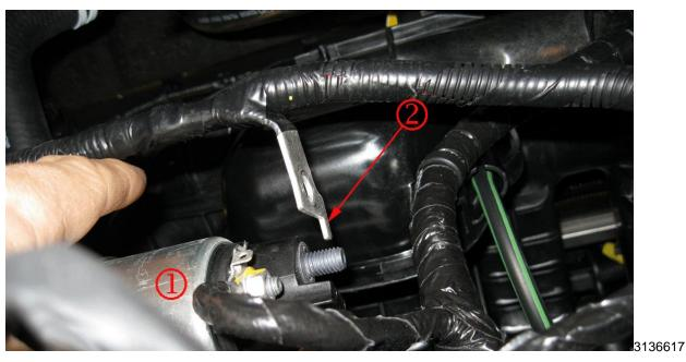
4. Remove the positive battery cable fastener and the positive battery cable terminal (2), from the starter solenoid (1).
