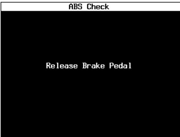
21. The ABS Check screen will instruct you to release the brake pedal.
