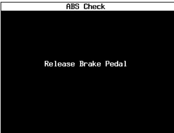
11. The ABS Check screen will instruct you to release the brake pedal.
