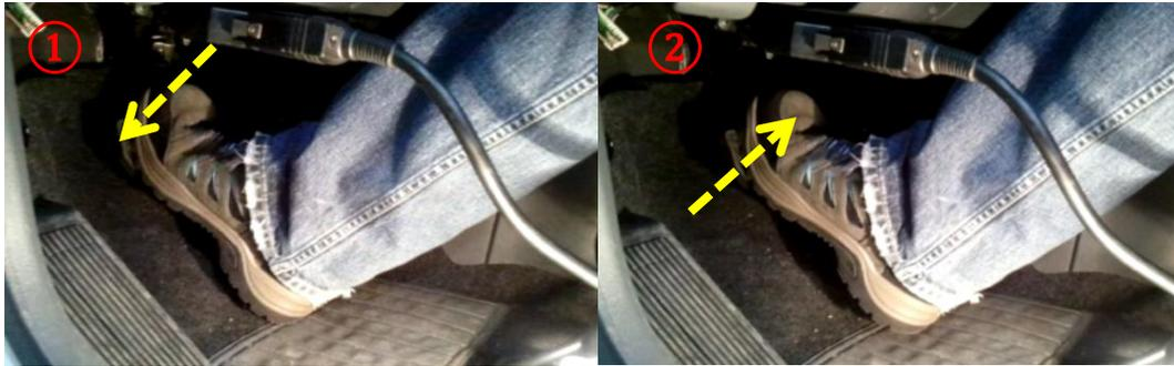
With the valve open, the pedal will drop for 2 seconds. With the motor pumping, the pedal will push back for 3 seconds.
