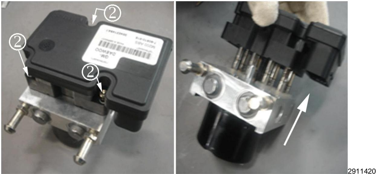
19. Remove the HCU from EBCM. (ABS: 3 bolts, ESC: 4 bolts).
