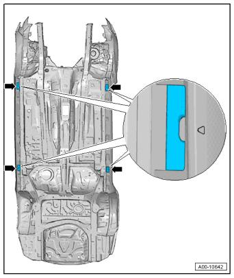
Position the lift pads on the plastic mounts (♠) found on the underbody.
