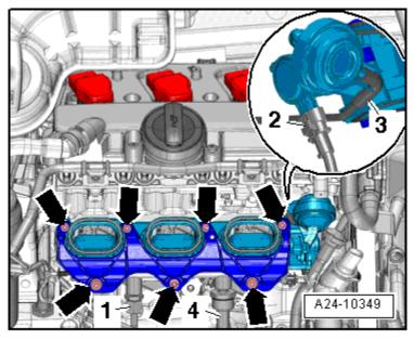
ComponentNmTighten bolts and nuts (➡) diagonally in stages10
