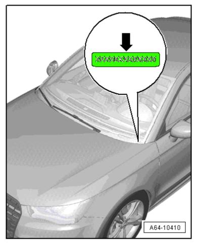
The VIN  $(\clubsuit)$  is on the left side of the vehicle in the area of the windshield wiper mount. It is visible from the outside.
