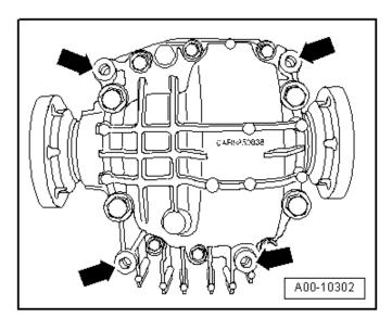
The 0BC final drive housing has four threaded holes (➡) used for attaching the cross member. An additional threaded hole under the flange/driveshaft attaches the final drive to the subframe.
