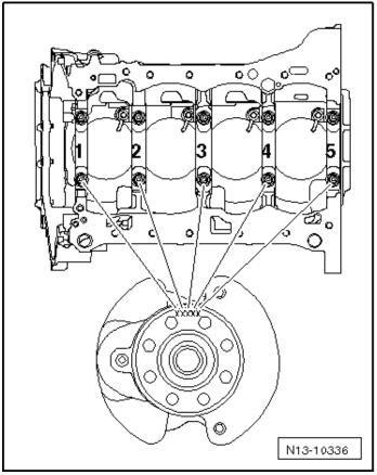
The identification on the crankshaft is for the lower bearing shell. Note the letter and match it to the color identification in the table.
