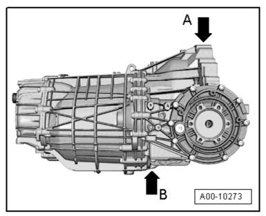
Transmission code letters and transmission serial numbers can be found on the top (A) and on the bottom (B) of the transmission housing.
