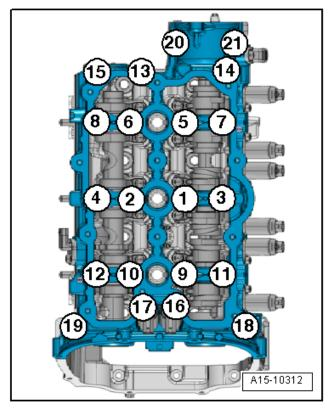
NOTE: The left cylinder head camshaft guide frame is shown. The right cylinder head camshaft guide frame is identical.
