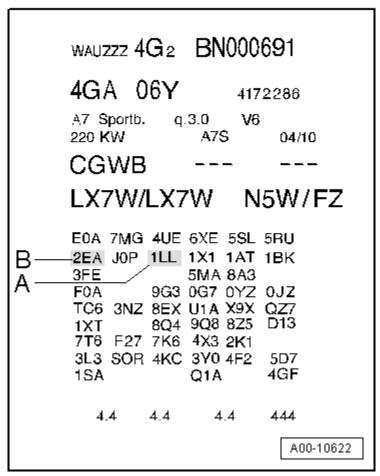
The brake system installed in a vehicle is indicated on the vehicle data label by the Production Relevant No. (PR No.) (A and B). Data label allocation, refer to the Electronic Parts Catalog (ETKA).
