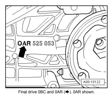
NOTE: 0AR is always on the rear final drive housing. The changes to the housing are what differentiate the 0BC final drive from the 0AR final drive.
