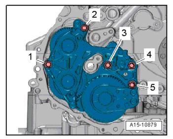
Tighten the bolts diagonally in the sequence -1 to 5- to 22 Nm.
