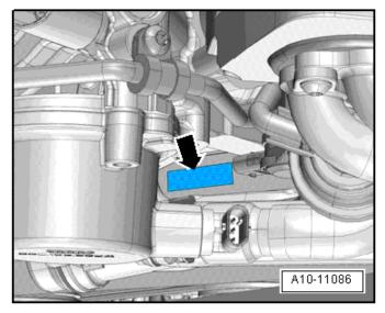
The engine number (engine code and serial number) is located on the top front of the cylinder block, below the right cylinder head (➡). Engine codes beginning with C are four-digit. The first 3 digits of the engine code indicate the displacement and the mechanical structure of the engine. The fourth digit describes the engine output and torque.
