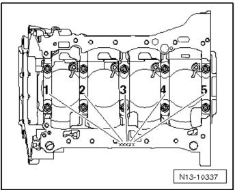
The cylinder block bearing shell identification is located either on the oil pan sealing surface or on the top (transmission side) of the cylinder block.
