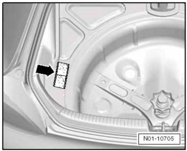
The vehicle data label (➡) is located on the left side of the spare wheel well. The vehicle data label is also in the customer's maintenance booklet.
