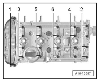
Loosen cylinder head cover bolts 1 through 6 in sequence.
