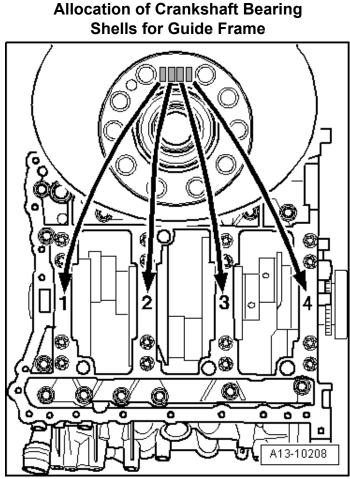
Bearing shells with the correct thickness are allocated to the guide frame at the factory. Colored dots on the sides of the bearing shells identify the bearing shell thickness. Allocation of the bearing shells to the guide frame is marked on the flywheel flange of the crankshaft by a row of letters. The first letter represents bearing 1, the second letter is for bearing 2, etc.
