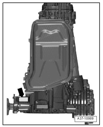
The transmission code letters are located on the data plate under the transmission. The  $\Rightarrow$  indicates the location of the type plate.
