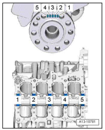
Bearing shells with the correct thickness are allocated to the guide frame in the factory. Colored dots on sides of bearing shells serve for identifying bearing shell thickness. The allocation of bearing shells to guide frame is identified by a letter on the front crankshaft flange, as shown in the illustration. The letter series begins with crankshaft bearing "5" (transmission side) and ends with crankshaft bearing "1" (belt pulley side).
