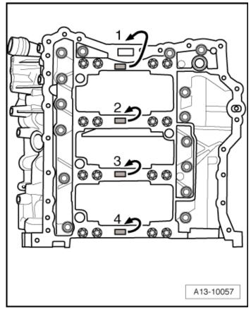
Bearing shells with the correct thickness are allocated to the cylinder block in the factory. Colored dots on the sides of the bearing shells identify the bearing shell thickness. Allocation of the bearing shells to the cylinder block is marked by a letter on the respective bearing on the guide frame.
