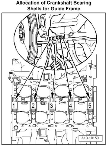
Bearing shells with the correct thickness are allocated to the cylinder block in the factory. Colored dots on sides of bearing shells serve for identifying bearing shell thickness. Allocation of bearing shells to cylinder block is marked by one letter each at left front on cylinder block (can be read from outside) as shown in the illustration.
