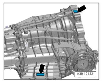
The transmission code letters are located on the transmission housing. The ➡ indicates the location of the type plate.
