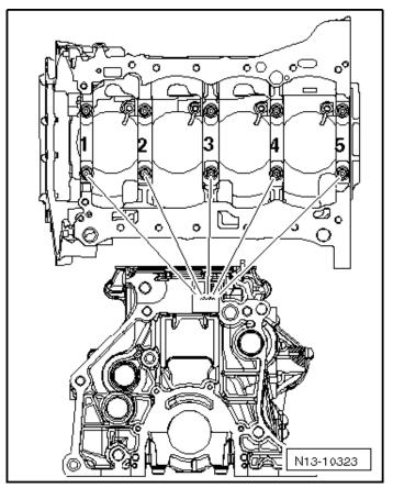
The identification on the cylinder block is for the upper bearing shell. Note the letter and match it to the color identification in the table.
