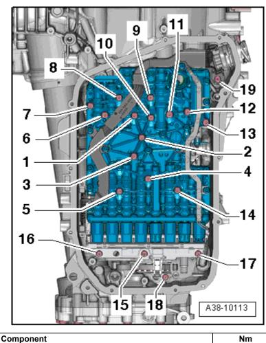
Mechatronic without Hydraulic Pulse Memory Tightening Specification
