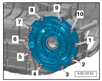
Replace bolts that are tightened to the specification.
