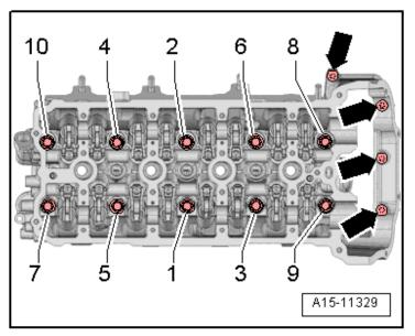
NOTE: Replace any bolts that were tightened with an additional turn. The cylinder head for cylinder bank 2 (left) is shown in the illustration.
