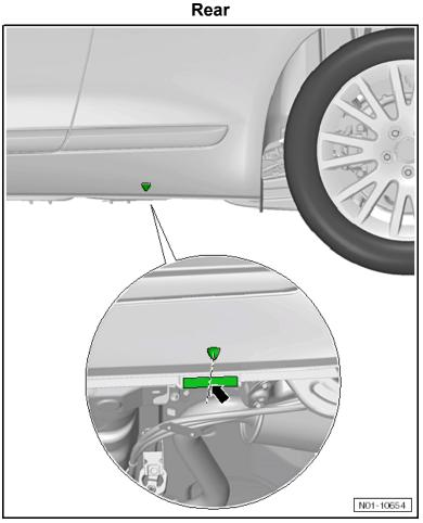
Position the support plate in the side member vertical reinforcement area (➡).
