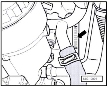
The engine number (engine code and serial number) (→) is located at the front of the engine/transmission joint. There is also a label on the toothed belt guard that shows the engine code and serial number. Engine codes beginning with C are four digit. The first 3 digits of the engine code indicate the displacement and the mechanical structure of the engine. They are stamped in the cylinder block, including the serial number. The fourth digit describes the engine output and torque.
