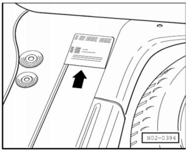
The vehicle data label (➡) is located in the left rear of the vehicle in the spare wheel well. The vehicle data sticker can also be found in the customer's service schedule.
