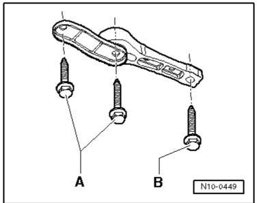
Secure the pendulum support to the transmission first and then to the subframe. To remove, first remove bolt B, then bolts A.
