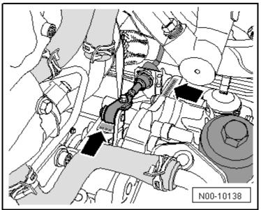
The transmission code letters can be found on the transmission near the selector lever cable  $(\Rightarrow)$  or under the transmission mount bracket.
