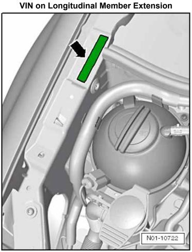
The Vehicle Identification Number (VIN) is located on the extension of the longitudinal member (➡).
