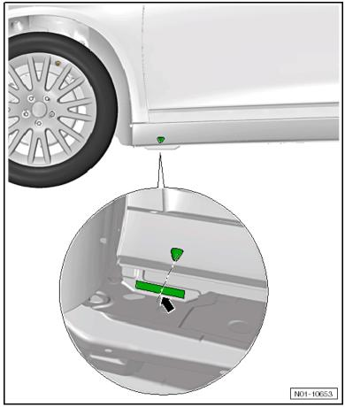
Position the support plate in the side member vertical reinforcement area (➡).
