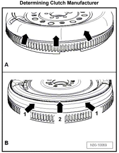
A) Round outer contour (➡) indicates a clutch manufactured by Sachs.
