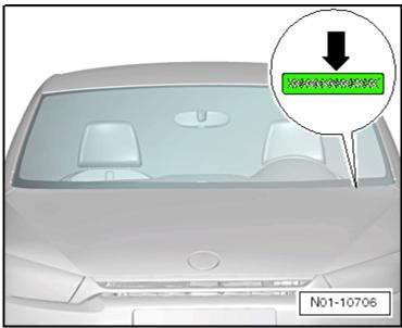
The VIN (➡) is on the left side of the vehicle in the area of the windshield wiper mount. It is visible from the outside.
