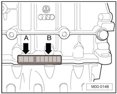
The engine code (A) and engine number (B) (serial number) are located on the rear side of the engine, above the cylinder block/ upper oil pan partition. The engine number consists of up to nine characters (alphanumeric). The first part (maximum of 3 letters) represents the engine code; the second (six digits) is the serial number. If more than 999,999 engines with the same engine code are produced, the first of the six characters is replaced with a letter.
