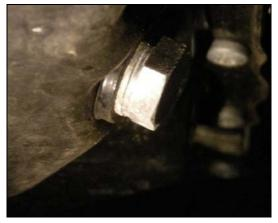
If the oil pan has a boss use part number: N 908 132 02 Drain plug w/seal
