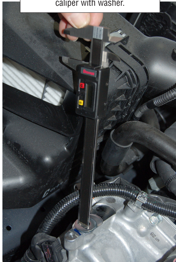
Measurement taken using digital caliper with washer.
