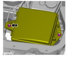
3. CAUTION: Make sure excessive force is not applied when repositioning the fuse box.
