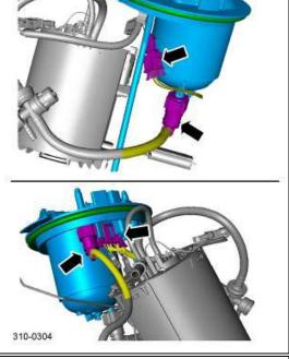
12. Remove and discard the blanking plug from the new fuel tank fuel outlet mounting flange.
