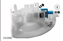
13. Remove and discard the clip from the new fuel tank fuel outlet mounting flange.
