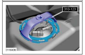
11. A NOTE: Hold the fuel tank fuel outlet mounting flange above the fuel tank aperture and allow any fuel within the fuel tank fuel outlet mounting flange to drain back in to the tank before attempting to withdraw it through the vehicle interior.
