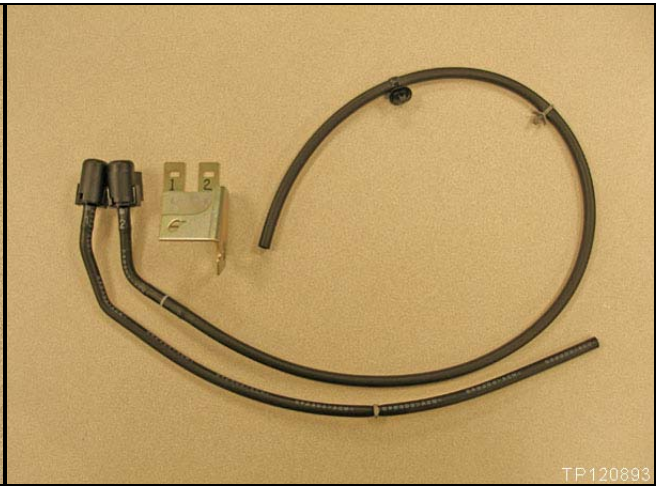
New (replacement) breather hoses and bracket
