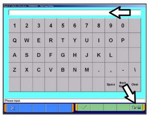
h. Click the icon in the lower RH corner of the screen to have MUT-III automatically read the VIN. If a message appears saying that the VIN cannot be input automatically, manually type the 17 digit VIN into the VIN field at the top of the page.
