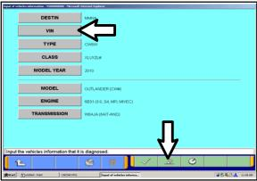
g. If the VIN or vehicle description displayed does not match the vehicle you are working on, click the eraser icon at the bottom of the page.
