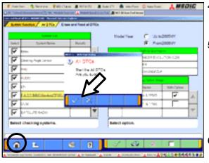
c. The list on the left side of the screen (System List) will have all selections checked. Do not change these selections. DTCs may be set if the vehicle is equipped with options that are unchecked.
