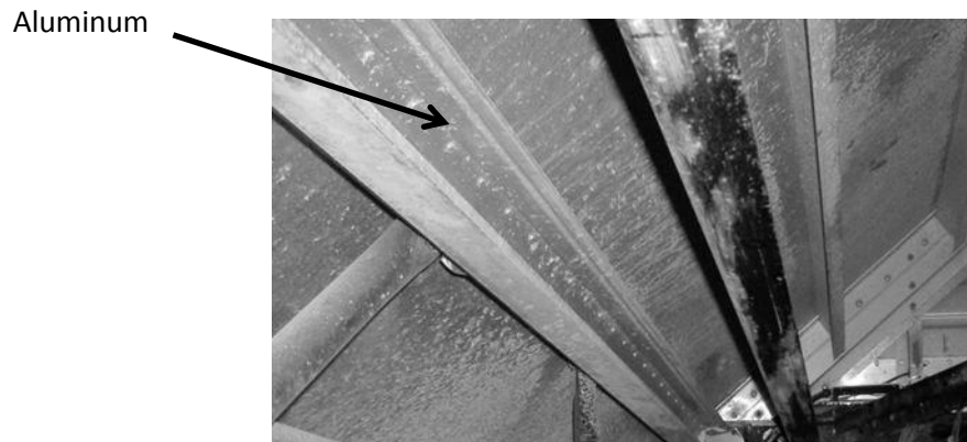
Figure 3: Early unit with Aluminum crossmember by landing gear.
