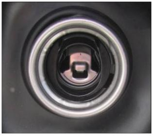
The mis-fuel inhibitor is designed to unlock and allow fueling only when a standard 24mm Diesel nozzle is installed on the filling pump at the fuel stations. The standard 24mm Diesel nozzle will fully engage the locking tabs on both the left and right side of the filler neck allowing the spring loaded locking collar to slide downwards, unlocking the restrictor flap allowing the nozzle to be inserted for fuel filling.
