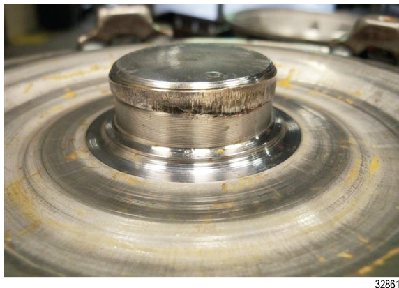
Figure 2. Torque Converter Pilot (Damaged)
