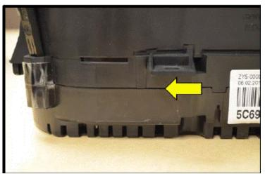
Inspect instrument cluster thoroughly to ensure both halves are fully seated and fastened together <arrow>.
