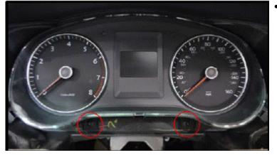
Remove the instrument cluster mounting bolts <circles>.
