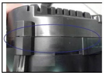
Since the lower housing does not fit properly with the upper housing, the buttons do not make contact when time and/or trip meter is being set.
