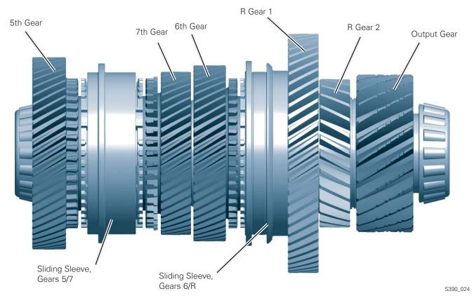
The following are located on output shaft 2:
