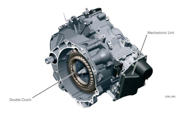
The dry double clutch has an extensive impact on the entire transmission concept. In comparison with the direct-shift transmission 02E, efficiency has been considerably improved. This improved efficiency makes a significant contribution towards lowering consumption and emissions.
