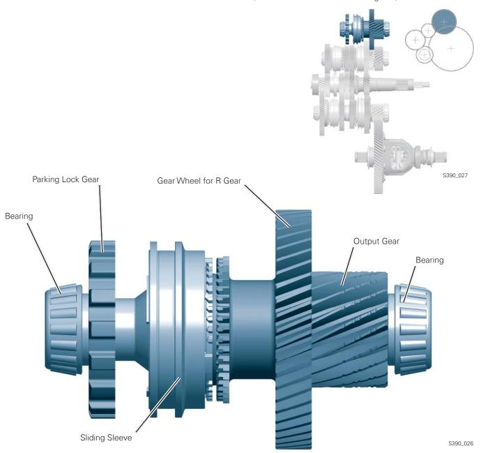
The following are located on output shaft 3:
