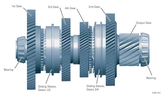
The following are located on output shaft 1:
