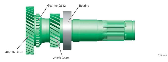
Drive shaft 2 is a hollow shaft. It is connected to K2 via splines. Drive shaft 2 is used to shift gears 2, 4, 6 and R. To record the transmission input speed, this shaft has the gear for G612 Transmission Input Speed Sensor 2.
