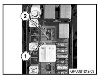
terminals shown in the illustration (2). The tool will activate the fan by connecting terminal 87 and 30 of the relay connector. For additional information refer to SI M04 14 12. The cooling of the engine requires aproximatly 2 hours.
