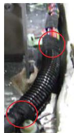
Photo 9: Tape both ends of corrugated tube
