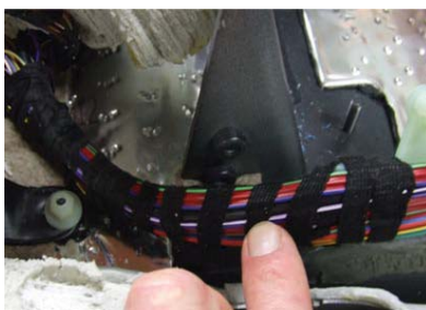
Photo 7: Lay harness in correct position and clips in correct orientation
