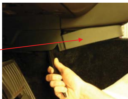
Photo 2: Trim tool to unclip and remove
