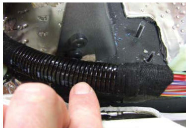
Photo 8: Corrugated tube to cover the damage points
