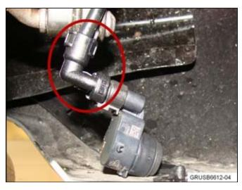
10. Install the "Protective Cap" as shown.
