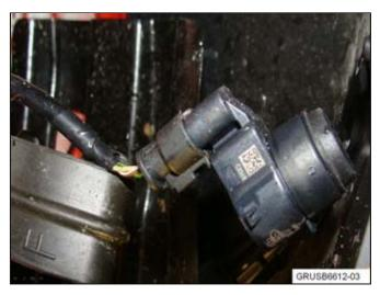
9. Uninstall the driver's side rear outer PDC sensor from the bumper mounting bracket.
