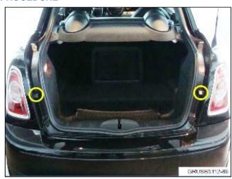
1. Open the tailgate and locate both lower rubber bump stops.
