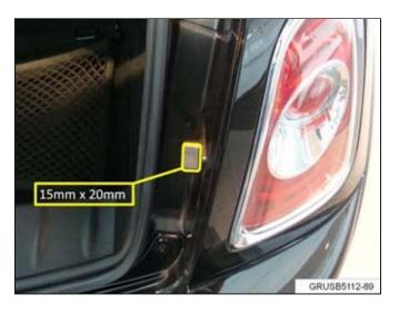
4. Clean off the mating surface of the bump stop with a suitable cleaner. Cut a new piece of sliding tape (83 19 9 407 798) approximately 15mm by 20mm and apply to the flat area of the rubber bump, as shown. Trim off any excess tape with scissors. Repeat the same repair procedure for the opposite side.
