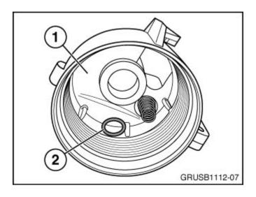
Engine oil filter housing (1) Rubber o-ring (2)
