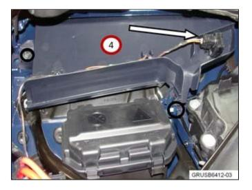
10. The fresh air intake cover (4) must be removed. Disconnect the sensor shown by the arrow and remove the two fasteners circled.
