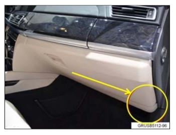
4. When reinstalling the trim, check the gap between the glove compartment and footwell trim. If the gap is larger than 2 mm, proceed to the next step.
