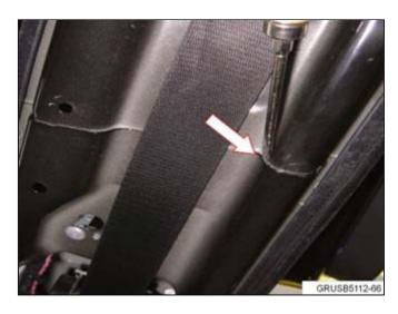
4. Insert a narrow screwdriver into the gap and gently pry outward to increase the gap, but no more than 0.3mm. Road test the vehicle to confirm the creak is eliminated.
