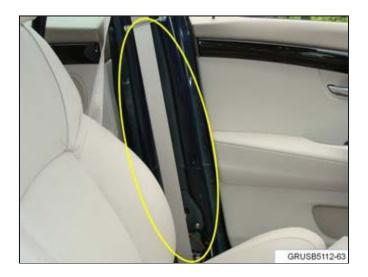
1. Using Repair Instructions 51 43 150, remove the B-pillar trim pieces from the affected side. Shown is the driver's side.
