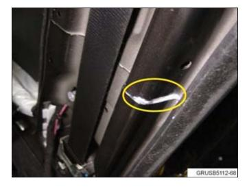
5. 5. Once the creak has been eliminated, fill the cavity with seam sealer and work it into the cavity to prevent future corrosion and sheet metal movement. Install the removed trim parts in the reverse order of their removal.
