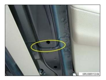
2. The area to be modified is where the two metal pieces of the Bpillar overlap.
