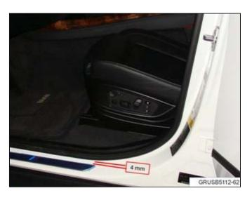
2. Remove the self-adhesive backing from the front sill strip and align the rear edge of the sill strip with the mark made earlier. Then position the trim parallel to the door sill at a distance 4mm-4.5mm away from the door opening, as shown. Apply the trim and press firmly to secure.
