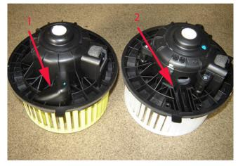
The design of the HVAC blower motor for these vehicles has been revised. The first design blower motor assembly has an integral cooling duct molded into the assembly (1). The second design blower motor assembly has a cooling port and uses a separate air duct that draws cooling air fro the lower section of the HVAC housing assembly (2).
