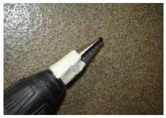
6. Using a single flute stepped drill bit, drill a 9/16-inch hole in the HVAC case lower half at the marked location. Do Not round-out the drilled
