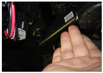
3. Place the new blower motor duct into position against the blower motor and HVAC case lower half as shown. Ensure it is in the installed position.
